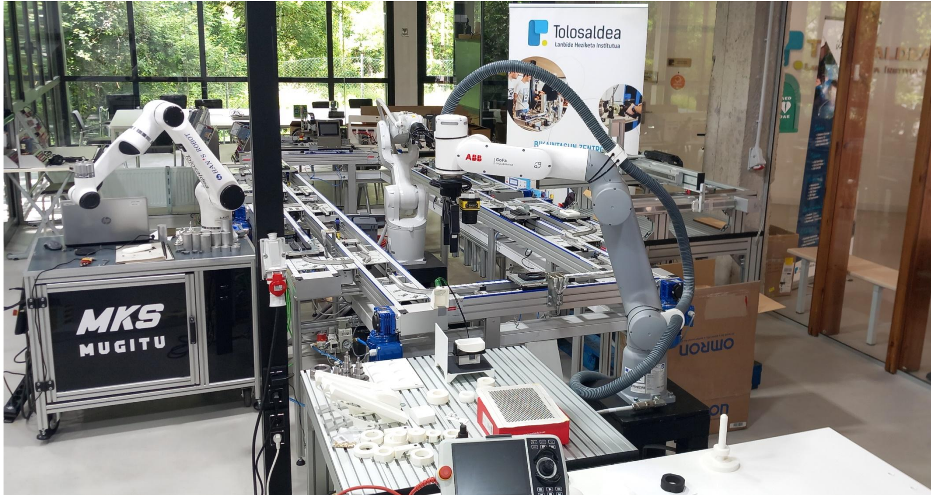
Our WS04 transfer line (6 workstations), where the final assembly and quality assurance take place
