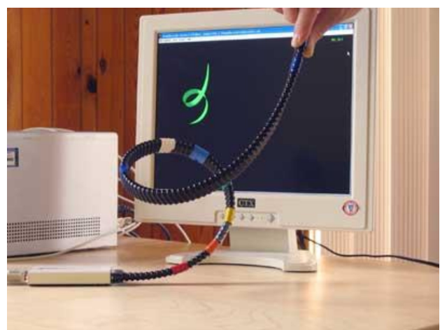
Figure 1: The TUI is a ShapeTape, a flexible that measures shape, position static and dynamic orientation [2].
